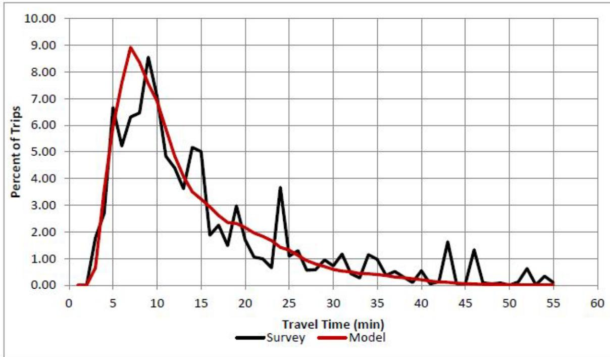
The trip distribution module [i.e., gravity model] is calibrated by adjusting friction factors until the two curves in the TLF plot match closely. Friction factors are model parameters/ coefficients within the gravity model equations that affect the distribution of trips between origins and destinations.
